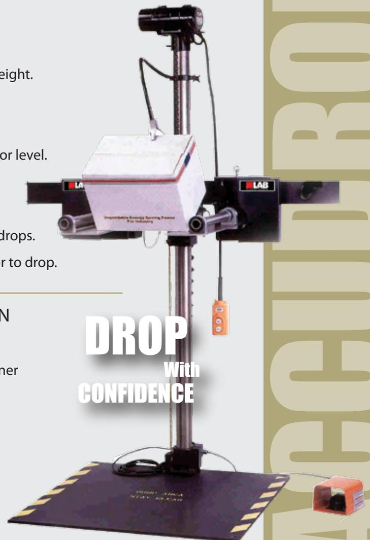
Dual Drop Leaf Release Mechanism
