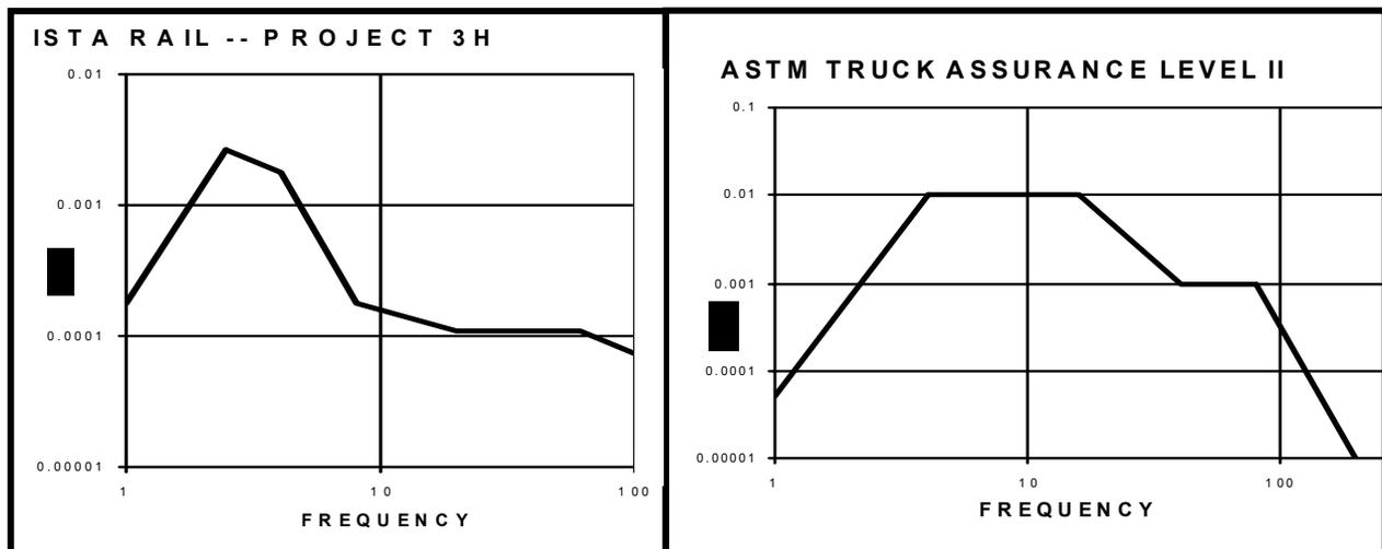
FIGURE 2: TYPICAL RANDOM SPECTRA (PSD PLOTS)
